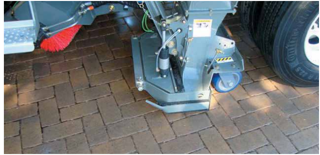
Vacuum Truck for Restorative Maintenance.
